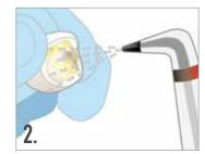
Air abrade internal surface, rinse, dry, and set aside. *NOTE: Contamination to the internal surface of the prosthesis will cause a decrease in bond strength. Keep area clean and free of phosphoric acid etch and saliva.*
